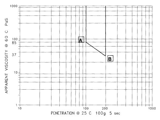
**Note:** Minimum viscosity at 60°C obtained from Cannon-Manning tube shall be on or above the A,B line corresponding to its penetration value.
